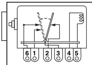
**MS2111** Replaces 221PH w/72 ohm coil. Used with NICS-78 non-incendive control system. Service part only.
