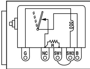
**518PH** Same as 517PH except allows for SWICHGAGE® and/or N.C. contacts to be wired "Closed Loop" (in series). Any contact open or SWICHGAGE® contact close in the circuit shunt trips the 518PH. Specify 12 or 24 VDC. Contacts 10 amps 24V. 14 amp fuse.
