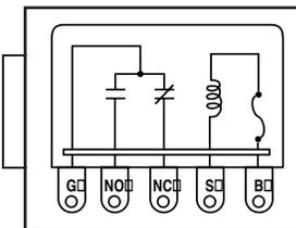
**R129A** A SPDT relay with 10 amp dry contacts. Specify 12 or 24 VDC. Contacts 10 amps 24 VDC. 14 amp fuse.
