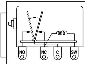
**822PH** Used in Murphy TR-assemblies as master disconnect. 24 VAC coil energizes when SWICHGAGE® contact closes to ground; breaks and makes circuit when tripped. Manual reset.
