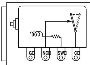
**521PH** Use with N.C. SWICHGAGE® or switches to ground magneto or CD ignition when tripped. Trip coil energized to run, de-energized to shutdown when N.C. contacts open. Specify 12 or 24 VDC. Contacts 10 amps 24 V.
