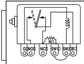
**518APH** Same as 517APH except allows for SWICHGAGE® and/or N.C. contacts to be wired "Closed Loop" (in series). Any contact open or SWICHGAGE® contact close in the circuit shunt trips the 518APH. Specify 12 or 24 VDC. Contacts 10 amps 24V. 14 amp fuse.
